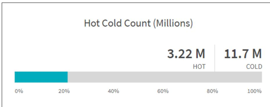
The Hot Cold Count graph displays the number of inodes (in millions) that are hot or cold in XCP NFS. In XCP SMB, this graph denotes the number of files that are hot or cold.
