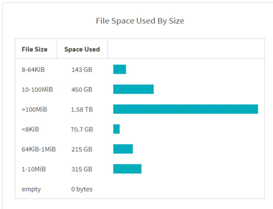
The File Space Used by size graph displays the number of files in different file-size ranges. The File Size column contains different file size ranges and the Space Used column indicates the space used by each file size range.
