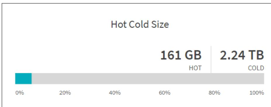
The Hot Cold Size graph displays the percentage of files that are hot and cold and the total size of the files in each category. The colored bar represents the hot data and the uncolored part represents the cold data. Criteria to define hot and cold data is based on access time only.
