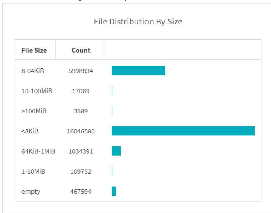
The File Distribution by size graph displays the number of files that are under the given file sizes. The File Size column contains the categories of file size and the Count column indicates the distribution of the number of files.
